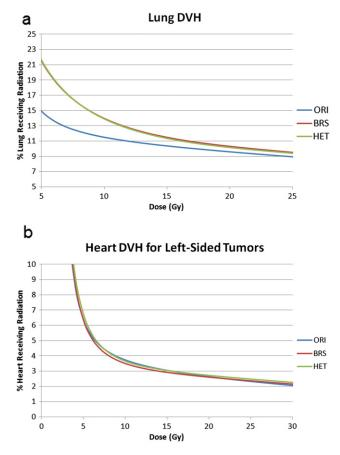
**Fig. 5.** (a) Dose-volume histograms comparing mean lung values of original (ORI), breast without IMP (BRS), and breast with IMP (HET) plans. (b) Dose-volume histograms comparing mean heart values of original (ORI), breast without IMP (BRS), and breast with IMP (HET) plans, where BRS and HET curves are superimposed.
